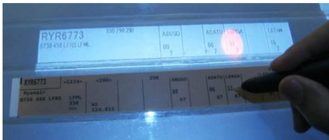
Figure 10: Virtual strip are projected on the stripboard. A controller points on a paper strip: the corresponding beacon is highlighted on the virtual strip.
