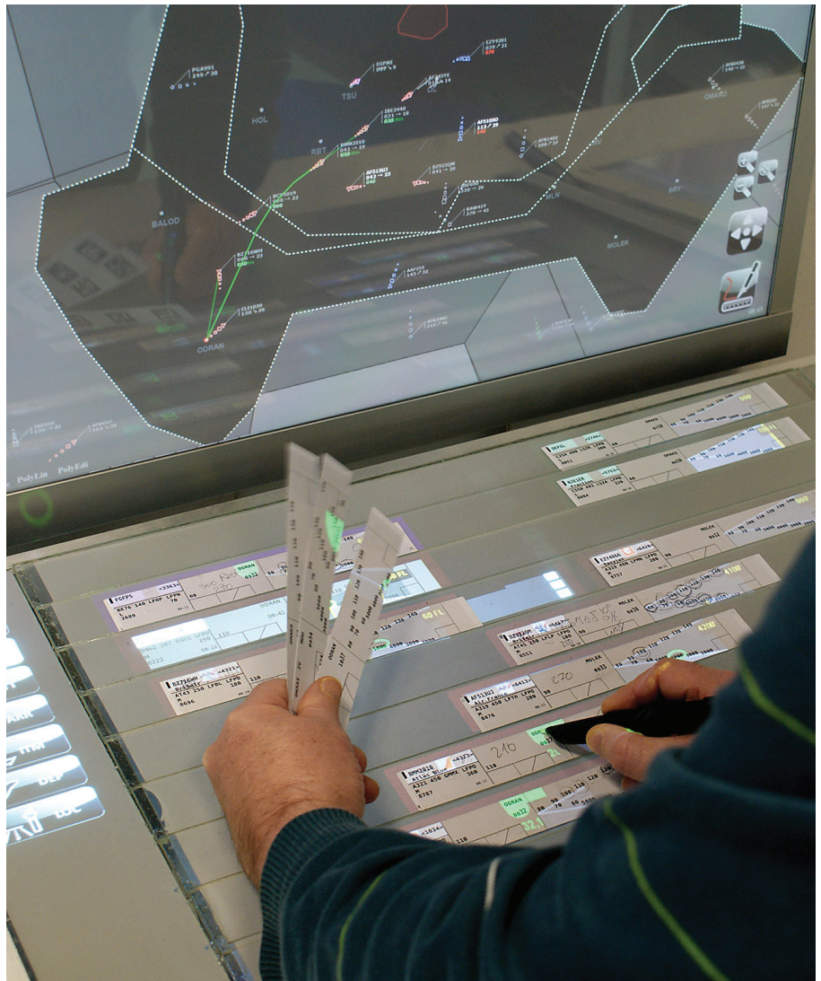
Strip'TIC mixes paper and electronic strips. The system tracks controller actions and pen input simultaneously (here filtering on a beacon started from an interaction with the paper strip).
