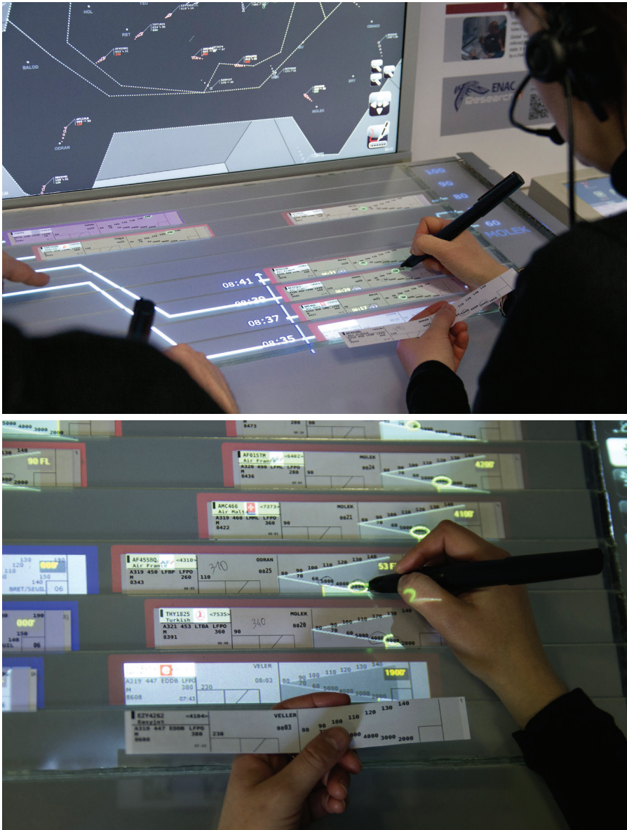
(Top) A controller collaboratively optimizes an arrival sequence, using a paper strip, numeric pen, and projected information. (Bottom) Free-hand writing and drawings convey key information.
