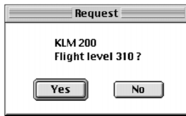
Figure 1: Proposing a new flight level to another air traffic controller: a rigid protocol
